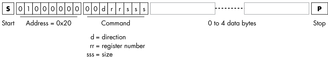
Figure 16-1: Peripheral write command
